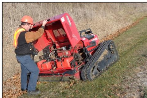
The wide opening hood provides access to the two removable fuel tanks. Marine style connections means fuel handling is fast and environmentally sound. Mechanical PTO drive and electrical cut height actuators minimize hydraulic connections and the potential for leaks and downtime.
