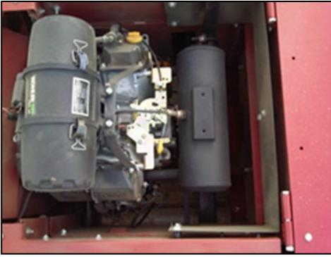
A 747 cc, twin cylinder air cooled Kohler engine – sized for productivity, chosen for fuel economy and reliability, provides power to the mower deck and the variable speed hydrostatic track drives.
