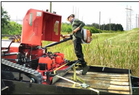
The bolt-on side panels permit easy service access when required. The hydraulic oil level sight glass is easy to see and the engine oil dipstick is conveniently located. A 12 volt remote battery boost terminal is positioned under the lockable hood. A battery master switch located 'out-of-sight' for added security.
